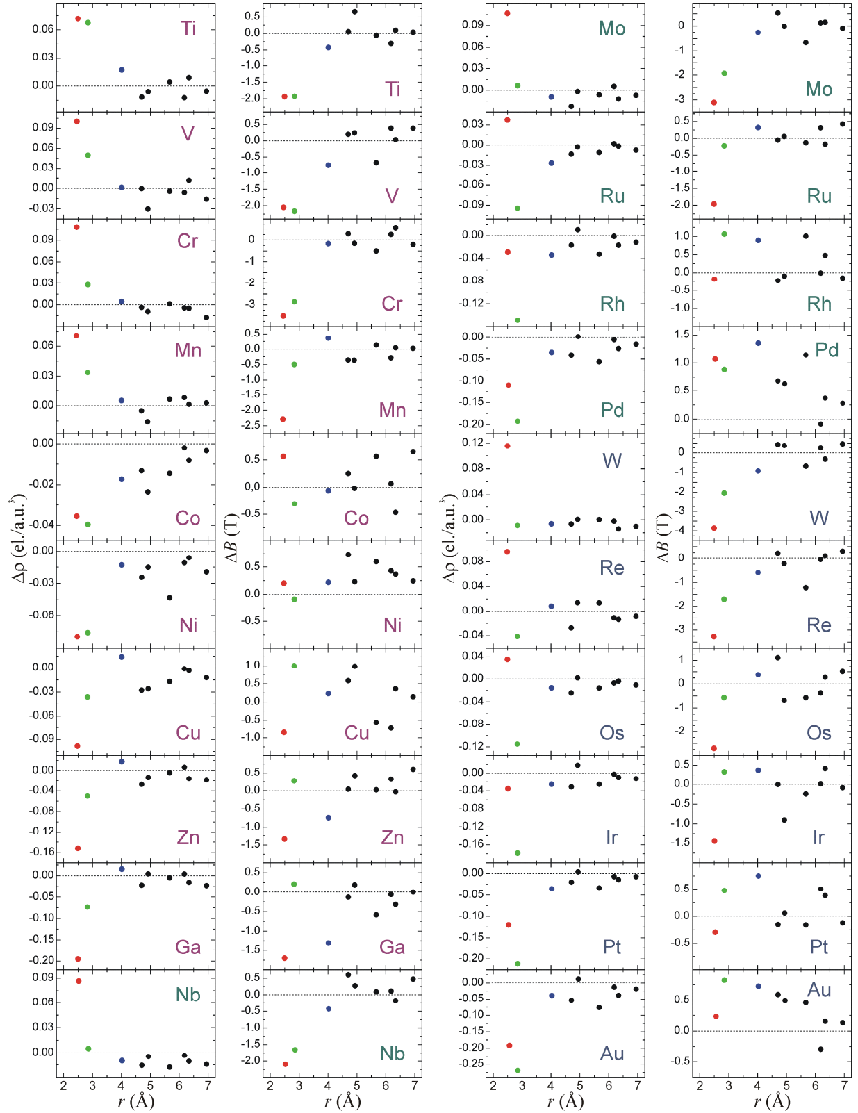
Figure 2 Calculated electron density perturbations \Delta\rho and spin density perturbations \Delta B plotted versus relaxed distance r from the impurity for various impurities. The zero level has been determined as described within text. Color distinguishes three first coordination shells. Figure is reproduced from Ref. [14].
